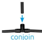
To conjoin the connectors, push the hose firmly into the unoccupied opening.
